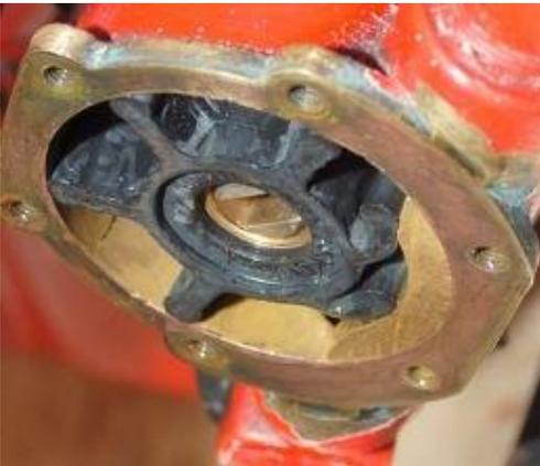
First close your seacock, (put a tag on the dash to remind you that it is closed) place your container under the pump to catch any errant screw that you may drop before it gets lost in the bilge, (Murphy's law) loosen all the screws and put aside. Don't be alarmed by any water that escapes from the housing.
