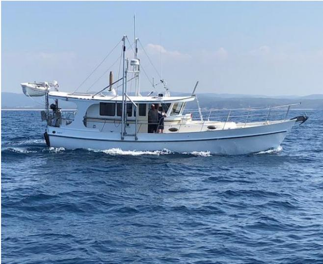
*Storm Boy II* is a custom built 42 ft fiberglass Trawler, the design was greatly influenced by Tasmanian trawlers and the final design and drawings were produced by Compu craft in Qld.
