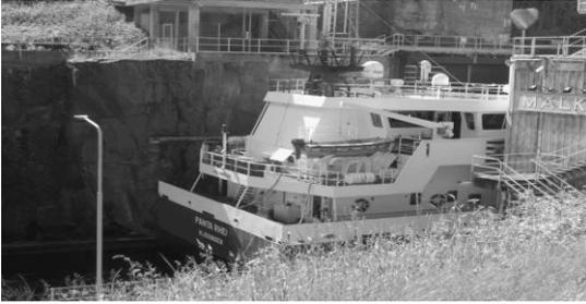
The canal was significantly overhauled and widened in 1963-68 before which there were 28 locks. The maximum dimensions for a ship transiting the canal are now: length 82.5m; beam 12.6m; draft 4.35m; air draft 24.5m. Those dimensions include ships of modest size carrying significant cargo, so the canal still carries considerable material, unlike many European canals that are now used
