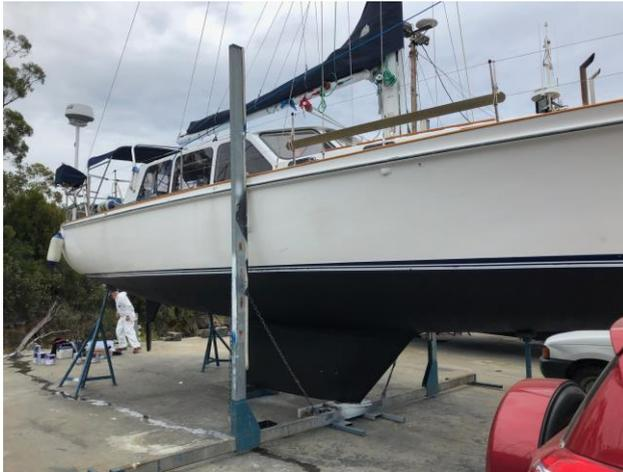
When the time came we slipped out of *Rubicon's* berth and motored around the corner to the lift and promptly with ease she was lifted out of the water and onto the hardstand. With water pressure cleaner in hand, gumboots on, Mike and myself took it in turns to clean off the minor weed growth, mussels and light covering of barnacles on the hull and keel. The task itself taking maybe an hour or
