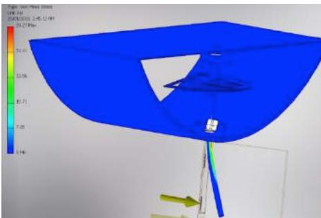
Figure 7. Potential bend in rudder post
