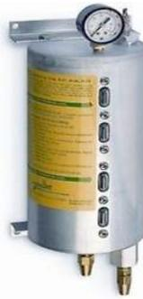
and in larger systems, especially where power auto-helms are employed, a pressurised reservoir is used to ensure that air is not sucked into the system, which in turn would cause sponginess (Compressed air entrapped in the lines when steering). These systems, once installed, providing all the connections are tight, will provide an extremely reliable and robust steering option.
