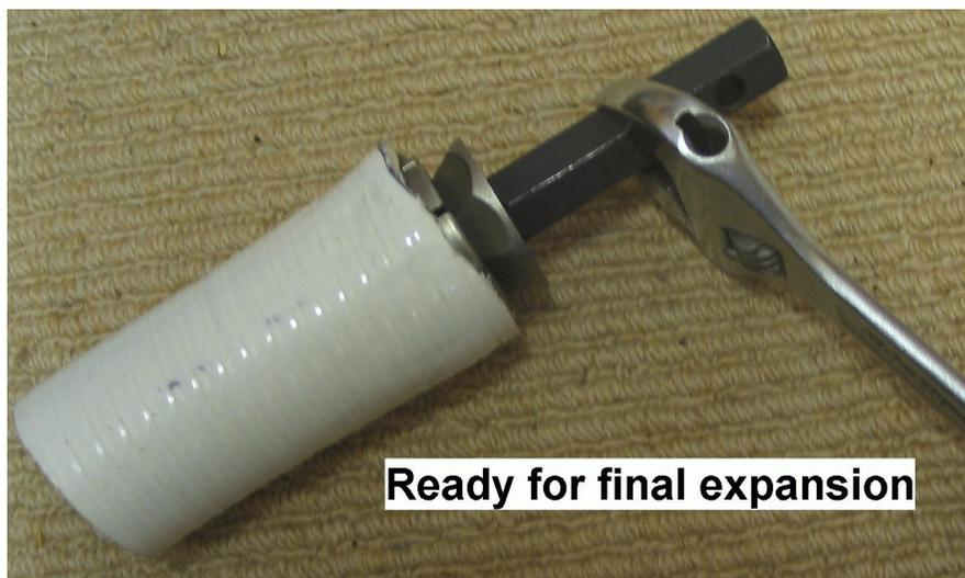
I'm not sure that it was necessary to warm the hose before pushing the tool in but it might take a few extra steps (push in, expand, contract, push in, ...) with cold pipe.
