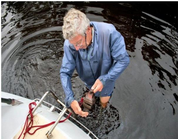
**Fitting the vice to the rudder, ready to winch it free**
