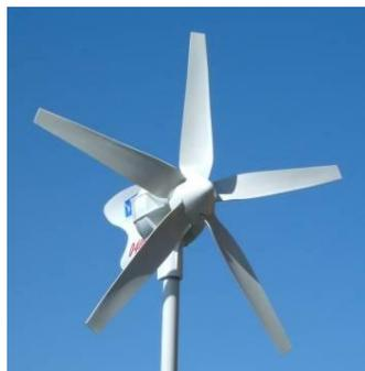
The D400 was easy to install, reusing most of our original generator tower. The tower needs to be robust as it weighs 17kg. It is a 5 bladed unit with a diameter of 1.1 metres - smaller than the KISS, but heavier. There is a need for a separate regulator and dump resistors which EoB sell. Power output really doesn't start until there is about 10kts of
