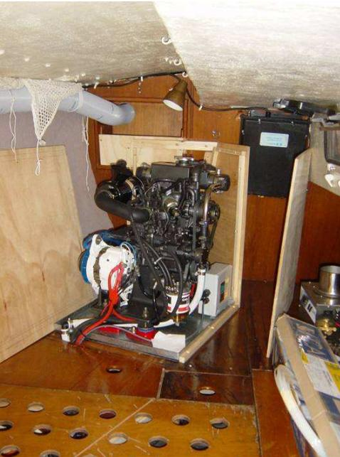
The diesel, named DAPO – short for **D**iesel **A**lternator **P**ower, is a 2 cylinder Kubota engine with a 210amp Balmar alternator, installed in a sound proof enclosure, which my Captain has made into a work of art. Each panel of the enclosure is interlocking and can be removed for ease of access for the diesel maintenance.
