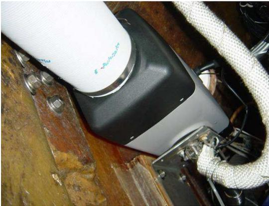
The natural position for the heating unit was the aft lazarette. Not much space left in there after the steering quadrant, hot water system, and port and starboard drogue rodes. Still Mike worked his magic once again and the unit was installed with the ex-
