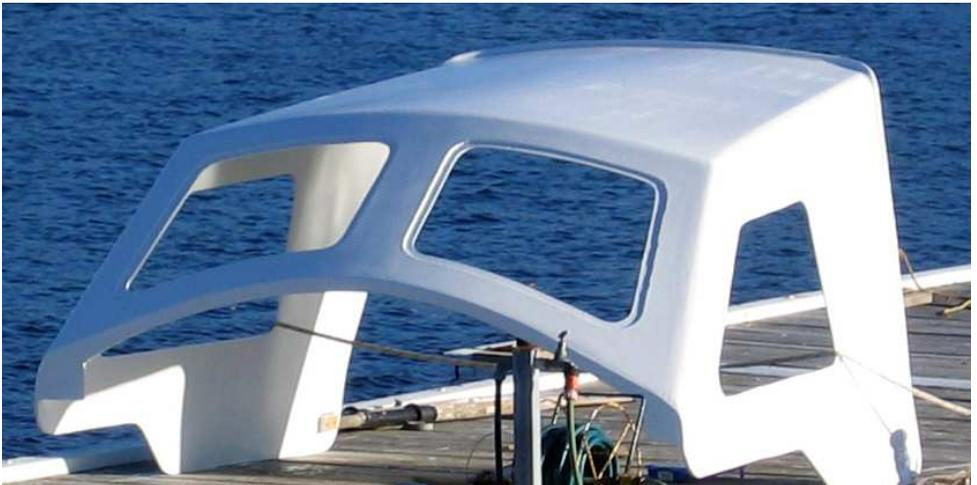
A length of retired jib sheet was used to form a drip lip along the roof edge overhang. This will also serve as a handgrip along the back edge of the dodger. It was continued down the sides to help channel water away from the cockpit. It was screwed on and then given several coats of resin and mat. Allow to dry.
