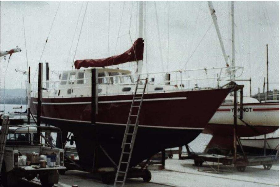
During the 1990s she had a complete refit which entailed fitting a pilothouse over the open centre cockpit, a complete interior refit, the removal of the reverse sheer, and the hull extended by 1 metre forming a rear cockpit, with outside steering. During this time she was also repowered with a Nanni 43h.p. diesel engine.
